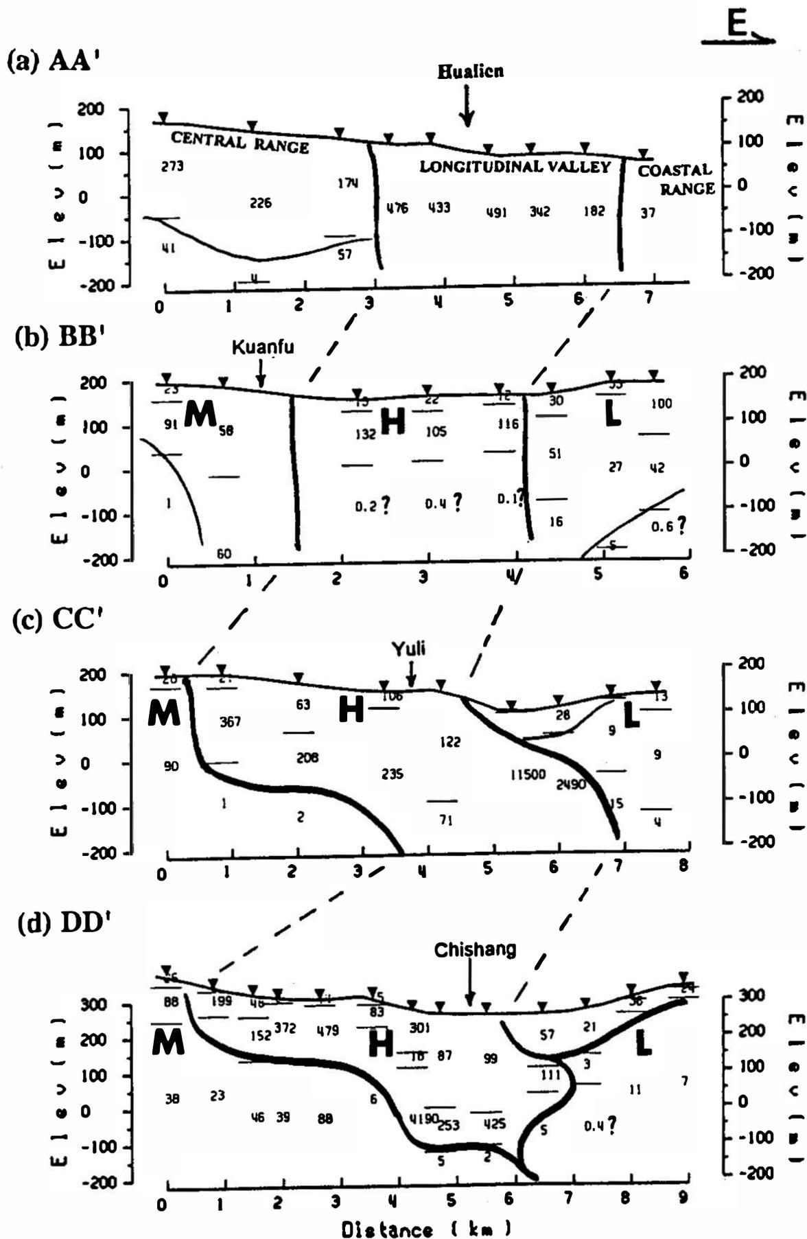
Fig. 10. Goelectric section of profiles AA', BB', CC' and DD' in Fig. 1a. The triangles indicate the sounding points. The interpreted positions of the layers and their resistivities in ohm-m are also shown. Dashed lines connect geoelectric boundaries among sections for reference.
