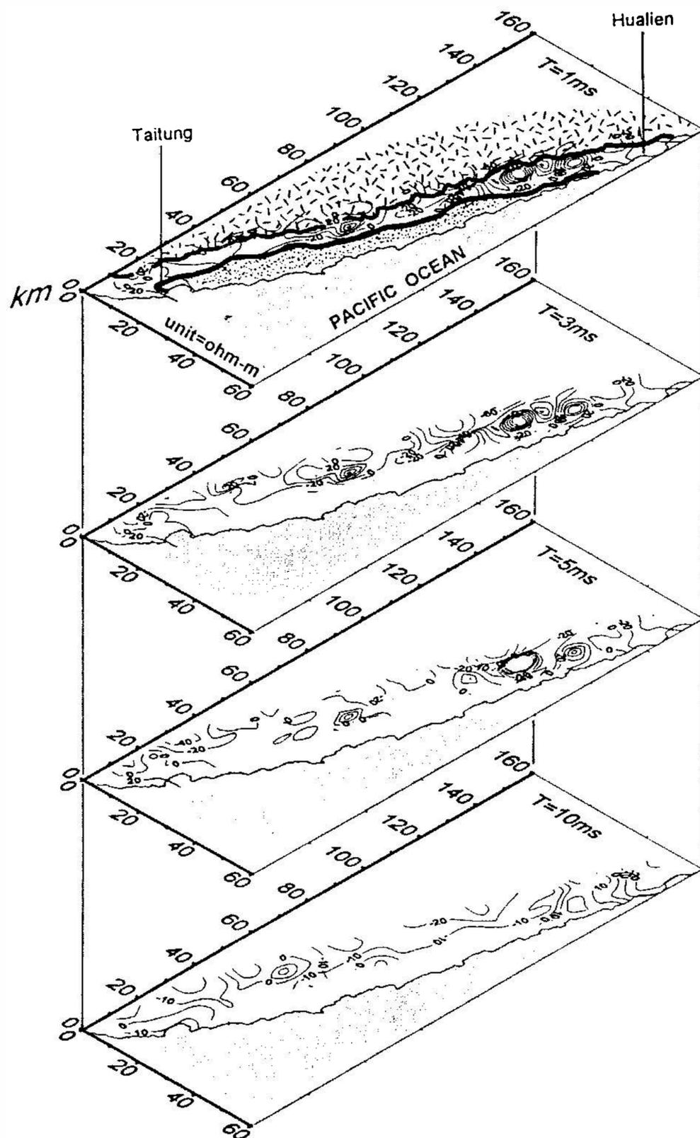
Fig. 7. Residual apparent resistivity contour maps at the delay times (a) 1 ms, (b) 3 ms, (c) 5 ms and (d) 10 ms after trend surface analysis.
