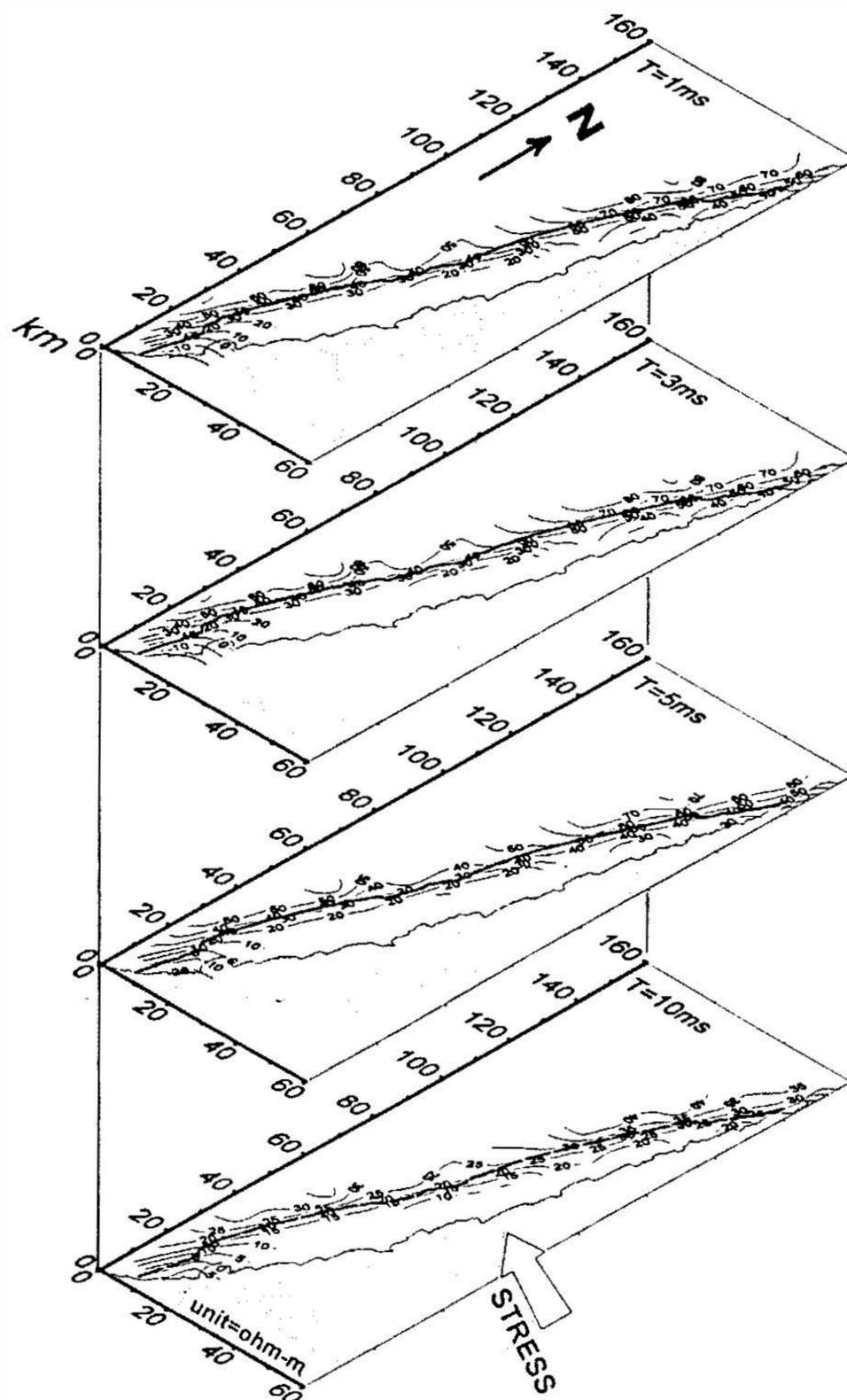
Fig. 9. 3D apparent resistivity regional map superimposed by the known suture line (bold line) of the Longitudinal Valley indicated in Fig. 2. A geoelectric suture line (approximately 25 ohm-m at 10 ms) between the two crusts is suggested from this study; the crusts being subject to a stress oriented in the NWW direction is also inferred.
