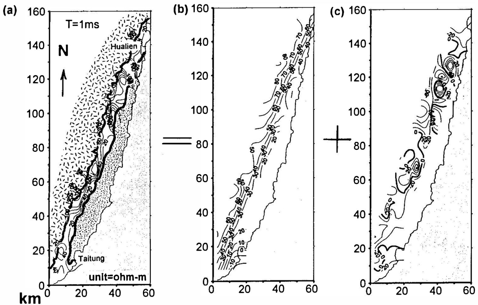
Fig. 6. (a) Resistivity contour map at the delay time of 1 ms in the Longitudinal Valley area. (b) First-degree trend surface. (c) Contoured residuals from the first-degree trend surface. Regional trend apparently shows the resistivities of the NNE trend which are hardly discernible on the observed resistivity map in (a).
