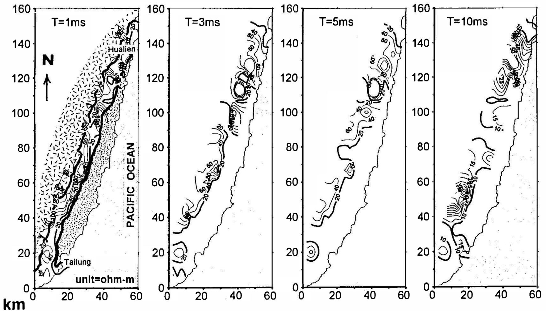
Fig. 5. Apparent resistivity contour maps of delay times  $T=1, 3, 5$  and  $10$  ms in the Longitudinal Valley, Taiwan. The bold lines (20-10 ohm-m) indicate low resistivity boundaries.
