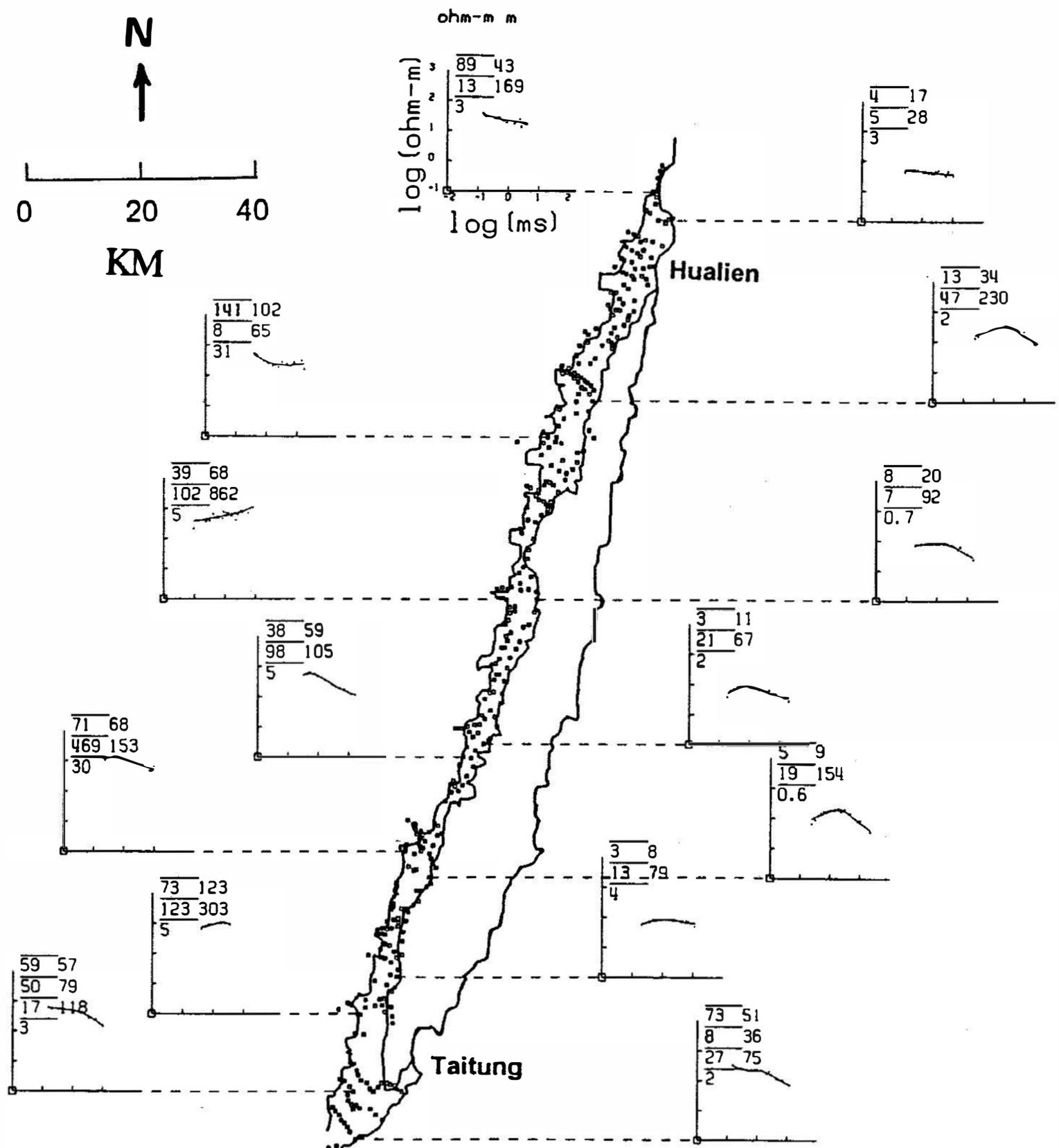
Fig. 4. Some typical field data and their inverted results of the TEM soundings in the Longitudinal Valley, Taiwan. In each sounding, dots are field data; the curve is the model value.
