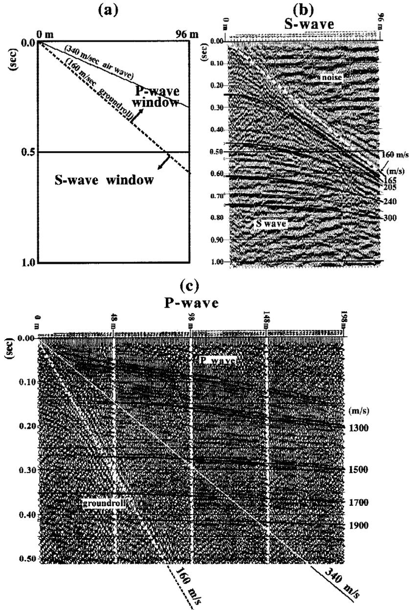
Fig. 8. The concepts leading to obtaining the P- and S-wave velocities in seismic reflection surveys. (a) gives the time windows where the S-wave (lower-left corner) and the P-wave (up-right corner) signals prevail, (b) and (c) respectively show the real data from which the velocities of the S- and P-wave are measured. The velocities are obtained according to the hyperbolic travel time assumption.
